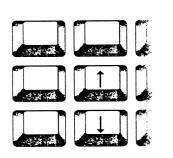
The Up Arrow / Down Arrow keys move the Menu Selection Bar and the Data Entry Form Field Selection Bar up or down one line.
